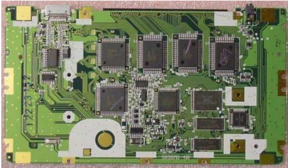
Component side of PCB
