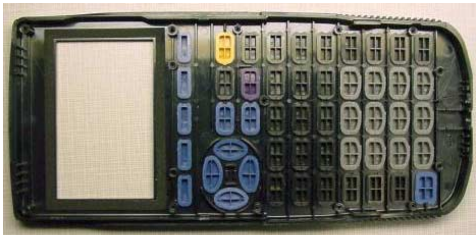
Inside front cover showing keycaps in place
