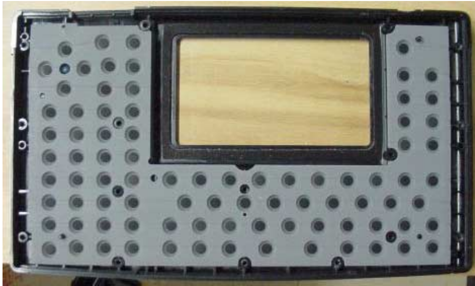
Key pad sheet, contact side
