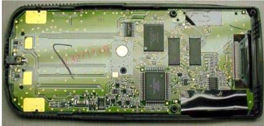
Component side of PCB with shield removed
